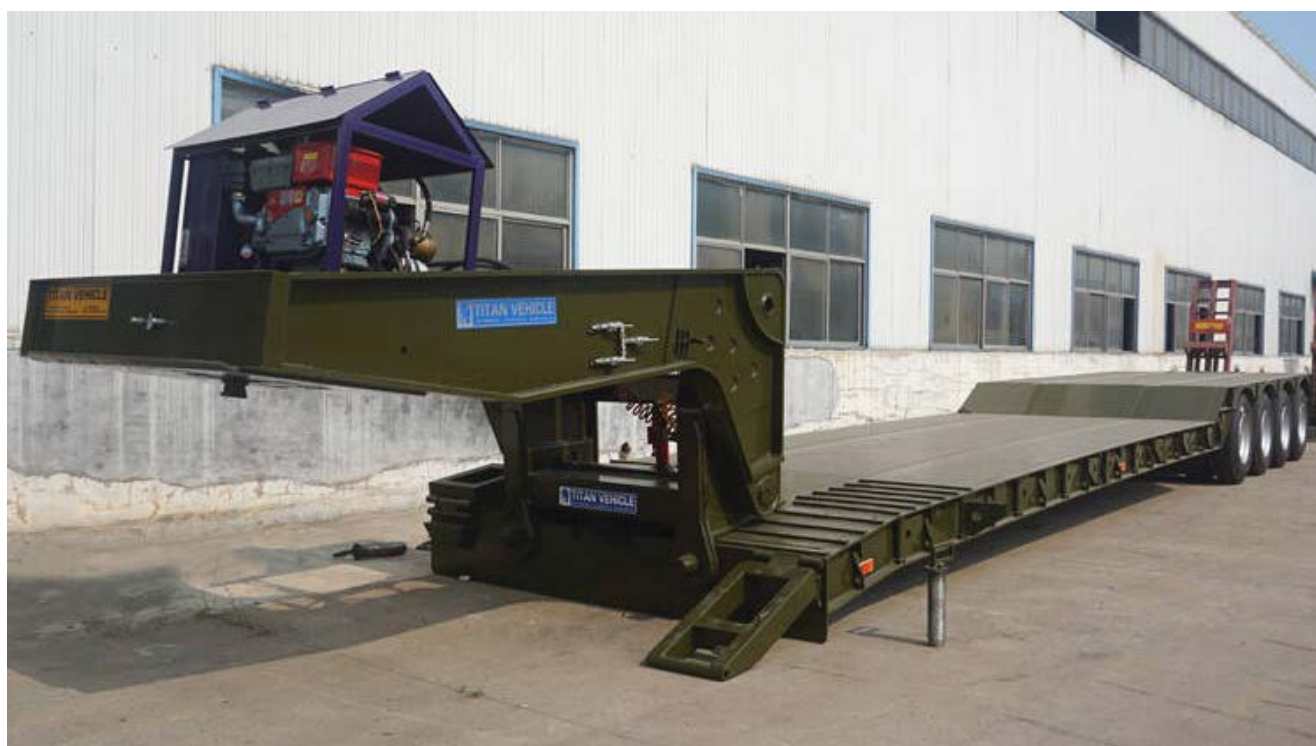
TITAN 4 axle 100 ton removable gooseneck semi trailer
