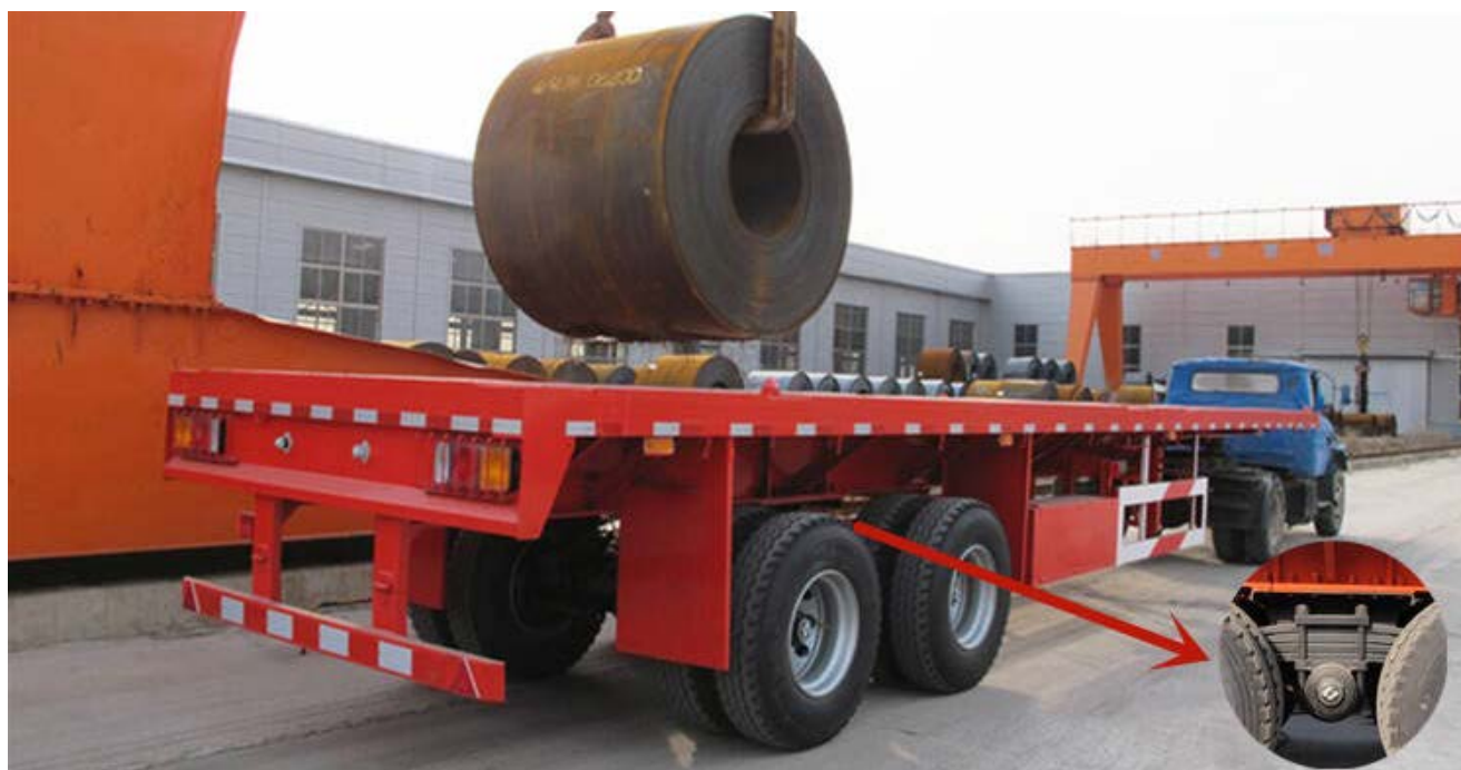
TITAN 2 axle flatbed semi trailer with bogie suspension
